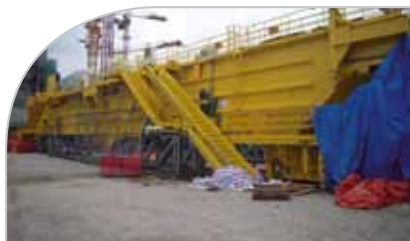
Polar crane delivery on site, Taishan (China)
