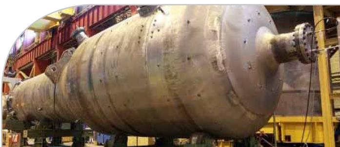
First FA3 steam generator during its secondary circuit hydrotest
