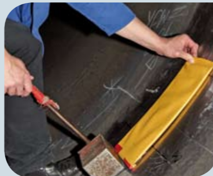
Placing a film for radio graphic testing
