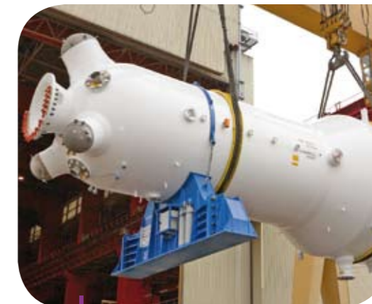
Shipment of a Steam generator for Saint-Lucie
